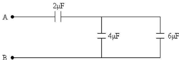
13) Three capacitors are connected as shown in Figure 21-17. What is the equivalent capacitance between points A and B? 13) \_\_\_\_\_
